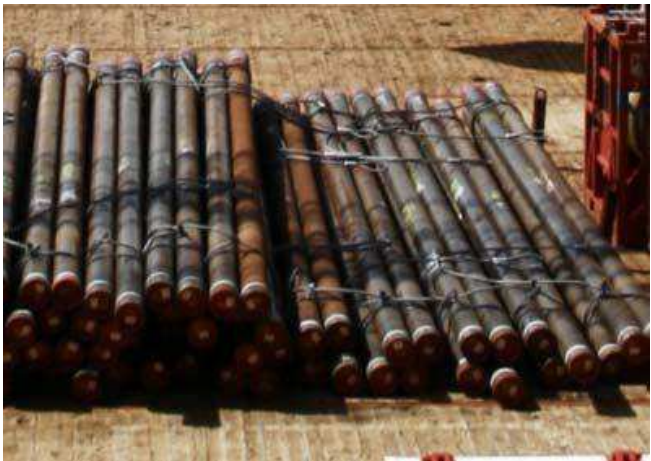
Figure 9 - B - 3 Casing (Dimensions range from 7" to 26")
