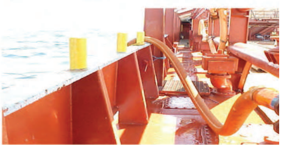
Floatation Hose Strings are available when bunkering to/from installations.
