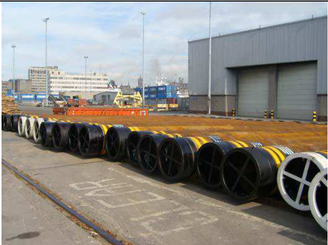
Figure 9 - B - 2 Conductors (Dimension 26" to 32")
